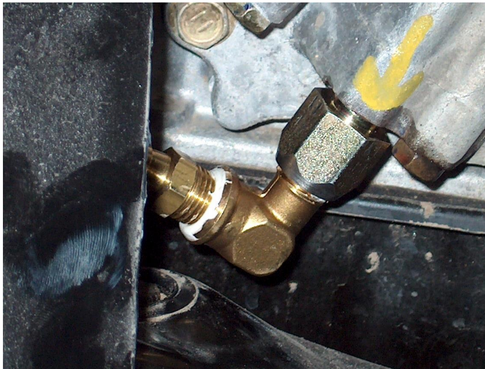
Arrow points to the port on the side of the transmission with adaptor plug installed.
